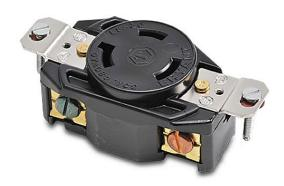
Bryant industrial heavy duty single locking blade receptacle, 30A, 480 VAC, 1-phase, 2-pole, 3-wire, NEMA L8-30, nylon molded housing, black.
