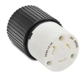
Bryant industrial heavy duty locking blade connector, 20A, 480 VAC, 1-phase, 2-pole, 3-wire, NEMA L8-20, accepts cord size 0.3-0.95in, nylon housing, black and white.
