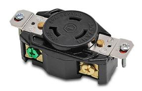
Bryant industrial heavy duty single locking blade receptacle, 20A, 480 VAC, 1-phase, 2-pole, 3-wire, NEMA L8-20, nylon molded housing, black.
