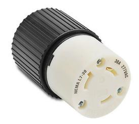
Bryant industrial heavy duty locking blade connector, 30A, 277 VAC, 1-phase, 2-pole, 3-wire, NEMA L7-30, accepts cord size 0.3-0.95in, nylon housing, black and white.
