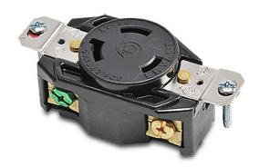
Bryant industrial heavy duty single locking blade receptacle, 30A, 277 VAC, 1-phase, 2-pole, 3-wire, NEMA L7-30, nylon molded housing, black.
