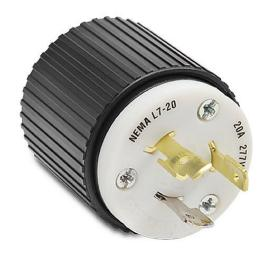
Bryant industrial heavy duty locking blade plug, 20A, 277 VAC, 1-phase, 2-pole, 3-wire, NEMA L7-20, accepts cord size 0.3-0.95in, nylon housing, black and white.
