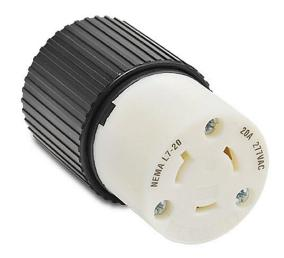
Bryant industrial heavy duty locking blade connector, 20A, 277 VAC, 1-phase, 2-pole, 3-wire, NEMA L7-20, accepts cord size 0.3-0.95in, nylon housing, black and white.
