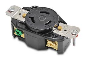
Bryant industrial heavy duty single locking blade receptacle, 20A, 277 VAC, 1-phase, 2-pole, 3-wire, NEMA L7-20, nylon molded housing, black.
