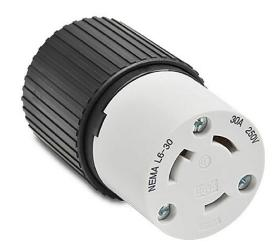
Bryant industrial heavy duty locking blade connector, 30A, 250 VAC, 1-phase, 2-pole, 3-wire, NEMA L6-30, accepts cord size 0.3-0.95in, nylon housing, black and white.
