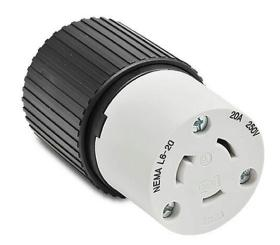
Bryant industrial heavy duty locking blade connector, 20A, 250 VAC, 1-phase, 2-pole, 3-wire, NEMA L6-20, accepts cord size 0.3-0.95in, nylon housing, black and white.
