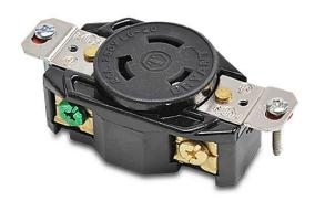
Bryant industrial heavy duty single locking blade receptacle, 20A, 250 VAC, 1-phase, 2-pole, 3-wire, NEMA L6-20, nylon molded housing, black.
