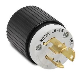
Bryant industrial heavy duty locking blade plug, 15A, 250 VAC, 1-phase, 2-pole, 3-wire, NEMA L6-15, accepts cord size 0.3-0.65in, nylon housing, black and white.
