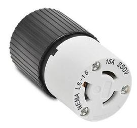
Bryant industrial heavy duty locking blade connector, 15A, 250 VAC, 1-phase, 2-pole, 3-wire, NEMA L6-15, accepts cord size 0.3-0.65in, nylon housing, black and white.
