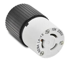
Bryant industrial heavy duty locking blade connector, 15A, 250 VAC, 1-phase, 2-pole, 3-wire, NEMA L6-15, accepts cord size 0.3-0.65in, nylon housing, black and white.
