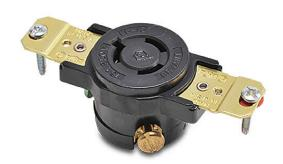
Bryant industrial heavy duty single locking blade receptacle, 15A, 250 VAC, 1-phase, 2-pole, 3-wire, NEMA L6-15, nylon molded housing, black.
