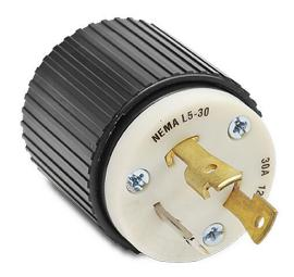
Bryant industrial heavy duty locking blade plug, 30A, 125 VAC, 1-phase, 2-pole, 3-wire, NEMA L5-30, accepts cord size 0.3-0.95in, nylon housing, black and white.
