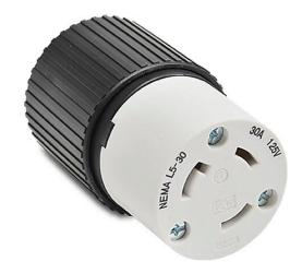
Bryant industrial heavy duty locking blade connector, 30A, 125 VAC, 1-phase, 2-pole, 3-wire, NEMA L5-30, accepts cord size 0.3-0.95in, nylon housing, black and white.
