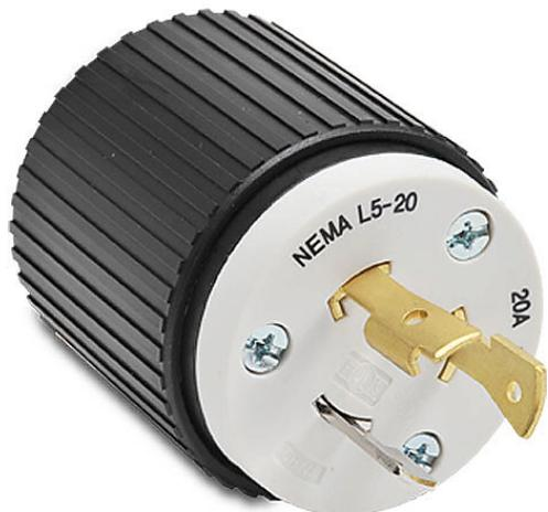
Bryant industrial heavy duty locking blade plug, 20A, 125 VAC, 1-phase, 2-pole, 3-wire, NEMA L5-20, accepts cord size 0.3-0.95in, nylon housing, black and white.
