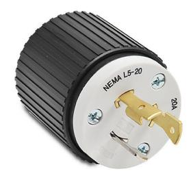
Bryant industrial heavy duty locking blade plug, 20A, 125 VAC, 1-phase, 2-pole, 3-wire, NEMA L5-20, accepts cord size 0.3-0.95in, nylon housing, black and white.
