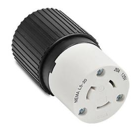
Bryant industrial heavy duty locking blade connector, 20A, 125 VAC, 1-phase, 2-pole, 3-wire, NEMA L5-20, accepts cord size 0.3-0.95in, nylon housing, black and white.
