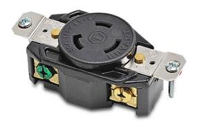
Bryant industrial heavy duty single locking blade receptacle, 20A, 125 VAC, 1-phase, 2-pole, 3-wire, NEMA L5-20, nylon molded housing, black.
