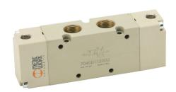
Metal Work pilot valve, 5-port (4-way), 2-position, double air pilot, 3/8in female NPT inlet(s), 3/8in female NPT outlet(s), 3/8in female NPT pilot(s), Cv=2.1.
