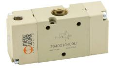
Metal Work pilot valve, 3-port (3-way), 2-position, N.O., single air pilot spring return, 3/8in female NPT inlet(s), 3/8in female NPT outlet(s), 3/8in female NPT exhaust(s), 1/8in female NPT pilot(s), Cv=2.1.
