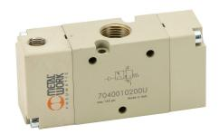
Metal Work pilot valve, 3-port (3-way), 2-position, N.C., single air pilot spring return, 3/8in female NPT inlet(s), 3/8in female NPT outlet(s), 3/8in female NPT exhaust(s), 1/8in female NPT pilot(s), Cv=2.1.
