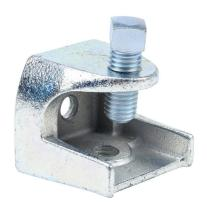
Minerallac screw-on beam clamp, 900 lbs. Package of 25. For use with flanges up to 7/8in and 1/2-13 threaded rod.
