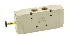
Metal Work solenoid valve, 5-port (4-way), 2-position, single solenoid spring return, 1/2in female NPT inlet(s), 1/2in female NPT outlet(s), 1/2in female NPT exhaust(s), Cv=4.6.
