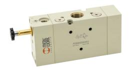
Metal Work solenoid valve, 3-port (3-way), 2-position, N.C., single solenoid spring return, 1/2in female NPT inlet(s), 1/2in female NPT outlet(s), 1/2in female NPT exhaust(s), 1/8in female NPT pilot(s), Cv=4.6.
