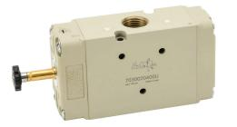
Metal Work solenoid valve, 3-port (3-way), 2-position, N.O., single solenoid spring return, 1/2in female NPT inlet(s), 1/2in female NPT outlet(s), 1/2in female NPT exhaust(s), Cv=4.6.
