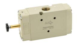
Metal Work solenoid valve, 3-port (3-way), 2-position, N.C., single solenoid spring return, 1/2in female NPT inlet(s), 1/2in female NPT outlet(s), 1/2in female NPT exhaust(s), Cv=4.6.
