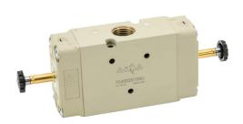
Metal Work solenoid valve, 3-port (3-way), 2-position, double solenoid, 1/2in female NPT inlet(s), 1/2in female NPT outlet(s), 1/2in female NPT exhaust(s), Cv=4.6.
