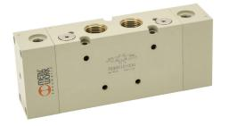
Metal Work pilot valve, 5-port (4-way), 3-position, center closed, double air pilot, 1/2in female NPT inlet(s), 1/2in female NPT outlet(s), 1/2in female NPT exhaust(s), 1/8in female NPT pilot(s), Cv=4.6.
