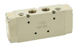
Metal Work pilot valve, 5-port (4-way), 2-position, double air pilot, 1/2in female NPT inlet(s), 1/2in female NPT outlet(s), 1/2in female NPT pilot(s), Cv=4.6.
