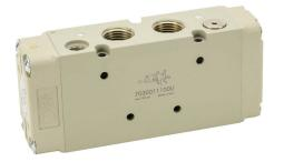
Metal Work pilot valve, 5-port (4-way), 2-position, single air pilot spring return, 1/2in female NPT inlet(s), 1/2in female NPT outlet(s), 1/2in female NPT exhaust(s), 1/8in female NPT pilot(s), Cv=4.6.
