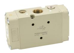
Metal Work pilot valve, 3-port (3-way), 2-position, N.O., single air pilot spring return, 1/2in female NPT inlet(s), 1/2in female NPT outlet(s), 1/2in female NPT exhaust(s), 1/8in female NPT pilot(s), Cv=4.6.
