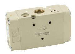
Metal Work pilot valve, 3-port (3-way), 2-position, N.C., single air pilot spring return, 1/2in female NPT inlet(s), 1/2in female NPT outlet(s), 1/2in female NPT exhaust(s), 1/8in female NPT pilot(s), Cv=4.6.
