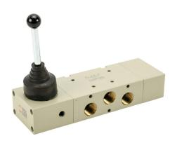
Metal Work pneumatic manual valve, 5-port (4-way), 3-position, center pressure, 90 deg hand lever, spring return, 1/2in female NPT inlet(s), 1/2in female NPT outlet(s), 1/2in female NPT exhaust(s), Cv=4.6.
