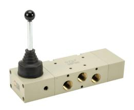
Metal Work pneumatic manual valve, 5-port (4-way), 3-position, center closed, 90 deg hand lever, spring return, 1/2in female NPT inlet(s), 1/2in female NPT outlet(s), 1/2in female NPT exhaust(s), Cv=4.6.
