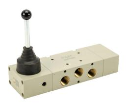
Metal Work pneumatic manual valve, 5-port (4-way), 3-position, center exhaust, 90 deg hand lever, spring return, 1/2in female NPT inlet(s), 1/2in female NPT outlet(s), 1/2in female NPT exhaust(s), Cv=4.6.
