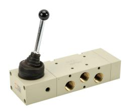
Metal Work manual valve, 5-port (4-way), 3-position, center pressure, 90 deg hand lever, detented, 1/2in female NPT inlet(s), 1/2in female NPT outlet(s), 1/2in female NPT exhaust(s), Cv=4.6.
