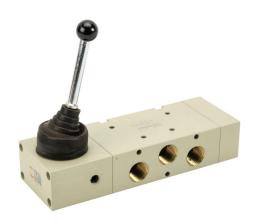
Metal Work pneumatic manual valve, 5-port (4-way), 3-position, center pressure, 90 deg hand lever, detented, 1/2in female NPT inlet(s), 1/2in female NPT outlet(s), 1/2in female NPT exhaust(s), Cv=4.6.
