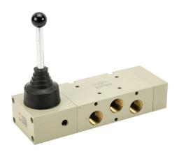
Metal Work pneumatic manual valve, 5-port (4-way), 3-position, center exhaust, 90 deg hand lever, detented, 1/2in female NPT inlet(s), 1/2in female NPT outlet(s), 1/2in female NPT exhaust(s), Cv=4.6.
