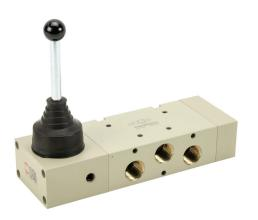
Metal Work pneumatic manual valve, 5-port (4-way), 3-position, center closed, 90 deg hand lever, detented, 1/2in female NPT inlet(s), 1/2in female NPT outlet(s), 1/2in female NPT exhaust(s), Cv=4.6.
