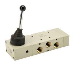
Metal Work pneumatic manual valve, 5-port (4-way), 2-position, 90 deg hand lever, detented, 1/2in female NPT inlet(s), 1/2in female NPT outlet(s), 1/2in female NPT exhaust(s), Cv=4.6.
