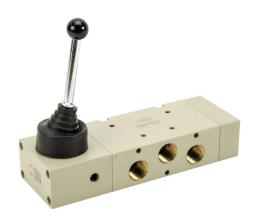
Metal Work pneumatic manual valve, 5-port (4-way), 2-position, 90 deg hand lever, spring return, 1/2in female NPT inlet(s), 1/2in female NPT outlet(s), 1/2in female NPT exhaust(s), Cv=4.6.
