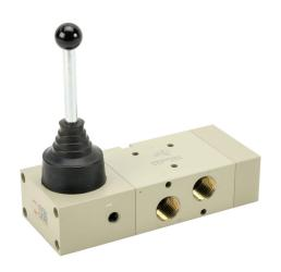
Metal Work pneumatic manual valve, 3-port (3-way), 2-position, 90 deg hand lever, detented, 1/2in female NPT inlet(s), 1/2in female NPT outlet(s), 1/2in female NPT exhaust(s), Cv=4.6.
