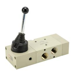
Metal Work pneumatic manual valve, 3-port (3-way), 2-position, N.C., 90 deg hand lever, spring return, 1/2in female NPT inlet(s), 1/2in female NPT outlet(s), 1/2in female NPT exhaust(s), Cv=4.6.
