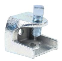
Minerallac screw-on beam clamp, 900 lbs. Package of 6. For use with flanges up to 7/8in and 1/2-13 threaded rod.
