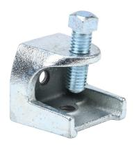
Minerallac screw-on beam clamp, 750 lbs. Package of 25. For use with flanges up to 3/4in and 3/8-16 threaded rod.
