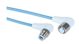
Murrelektronik connection cable, M12 right-angle male to M12 right-angle female, 4-pole, styrene-butadiene thermoplastic (TPE-S) jacket, ice blue, 16.4ft/5m cable length, IP65, IP68 and IP69K, suitable for food and beverage applications, FDA compliant.
