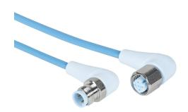
Murrelektronik connection cable, M12 right-angle male to M12 right-angle female, 4-pole, styrene-butadiene thermoplastic (TPE-S) jacket, ice blue, 9.8ft/3m cable length, IP65, IP68 and IP69K, suitable for food and beverage applications, FDA compliant.
