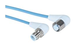
Murrelektronik connection cable, M12 right-angle male to M12 right-angle female, 4-pole, styrene-butadiene thermoplastic (TPE-S) jacket, ice blue, 3.2ft/1m cable length, IP65, IP68 and IP69K, suitable for food and beverage applications, FDA compliant.
