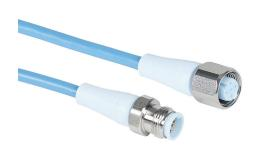
Murrelektronik connection cable, M12 axial male to M12 axial female, 5-pole, styrene-butadiene thermoplastic (TPE-S) jacket, ice blue, 3.2ft/1m cable length, IP65, IP68 and IP69K, suitable for food and beverage applications, FDA compliant.
