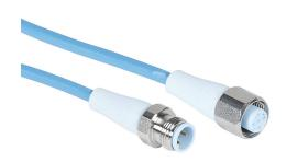
Murrelektronik connection cable, M12 axial male to M12 axial female, 4-pole, styrene-butadiene thermoplastic (TPE-S) jacket, ice blue, 16.4ft/5m cable length, IP65, IP68 and IP69K, suitable for food and beverage applications, FDA compliant.
